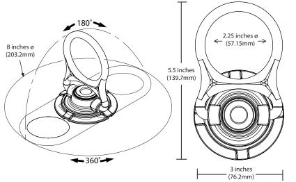
Tensile Strength (UTS): 5,000-lbf (22kN)
